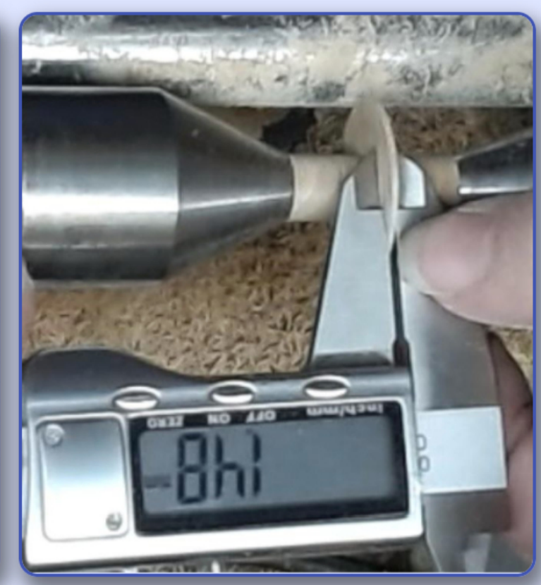
Photo 9 - Using a Vernier
