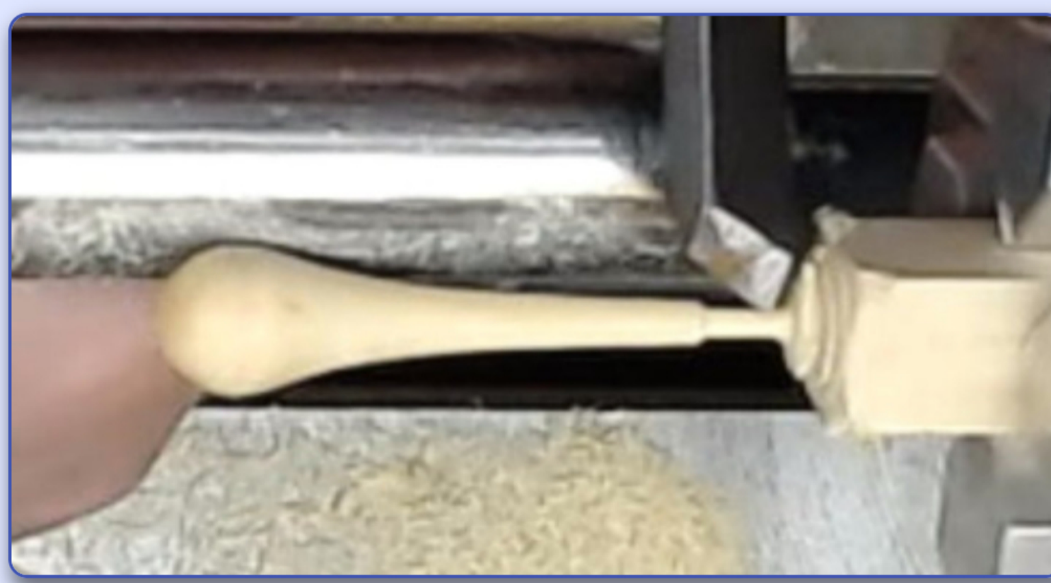
Photo 5 - Finished Pendant Before Parting Off
