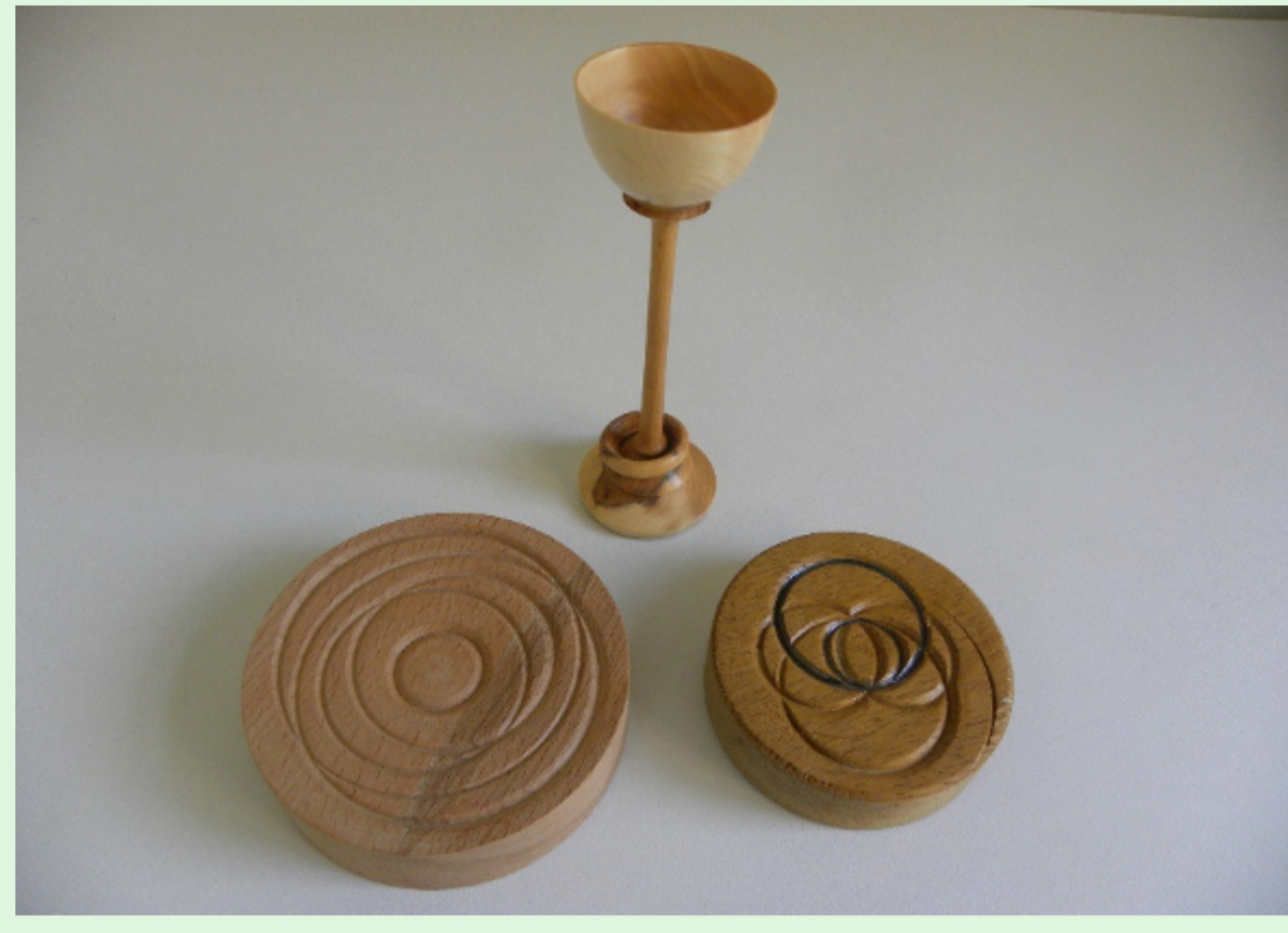
Photo 7 - Goblet with Captive Ring and Off-Centre Turning
