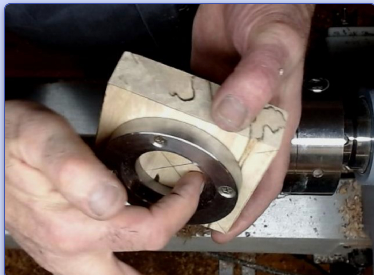
Photo 9 - Showing faceplate ring attached
