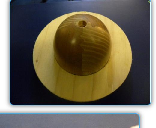
The turning of the spindle is not easy to describe but I have added a drawing at the end of the write up for you. This was sanded and polished using 120 to 320 Demo finish but if competition would go up to at least 600 if not higher.
