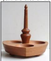
circle of the dish or bowl centres. Two 120° apart and the third on the straight line produced opposite one of them, accuracy is important. The stand I am making is from a 150mm diameter blank, so my jig is about 30mm greater in diameter to allow space for the counterweights.
