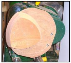
The underside of the base can now be screwed to the jig using hole 4 on the jig
