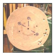
These are almost on the edge of the jig, but just far enough in to be secure. The counterweights used here are strips of lead, rolled and bolted to the back of the jig. The size and number of strips used will depend upon the set up. The weight of lead is easily adjustable, so trial and error to get it right is possible.
