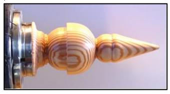
Now is the time to cut across to form the base. I start by going in about 10mm with a parting tool, leaving 1mm or so of wood to remove from the base with the toe of a skew chisel. I remove this millimetre, cutting square to the lathe.
