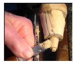
The tops may be formed to any appropriate shape. Here I am using some small left over pieces of spalted beech glued onto some waste wood for chucking. The stoppers have been finished with a coat of cellulose sealer followed by two coats of melamine. They were rubbed down with 0000 grade steel wool between the coats.
