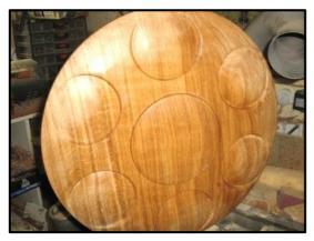
That's just about it for the turning. Here I've completed the six petals, sanded the piece and sprayed it with a coat of acrylic sanding sealer.
