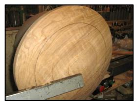
The piece is now mounted with that front spigot in the big chuck jaws. The back has been dished slightly, the 14½ inch line repeated on the back, six equally spaced radial lines marked (using the lathe's indexer) and another chucking spigot developed in the centre.
