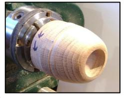
If the right size drill is not available, a drilled hole has to be finished this, or a similar, way. With the recess finished, the top part of the outside can be formed, the shape decided by the turner to suit requirements.
