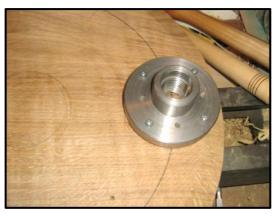
The 4 inch faceplate is then screwed round the six petal locations. I sighted the 14½ inch ring through two of the holes, the radial line through two others, and screwed it through the other four. Confession time. Notice that there is a small wedge to the left side of the faceplate in this picture - after all was said and done, I dished the piece too much and it fouled the lathe, so the wedge straightened it out for me. It's a learning curve!
