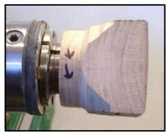
Hold the work and form a dovetail. This time I held it by friction hold, but there are various methods. The wood was an old oak fence post and has cracks where shown by the arrows. The cracked section I left on to form the jam chuck later on. (It could of course be made out of a separate piece of wood). The jaws of the chuck are holding the split wood, so the cracks should not present a problem. Just make sure they do not extend into the area of the finished article.
