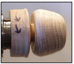
sanding over some of the finished work and refinishing as I finalise the underside on the jam chuck. Now part off the work. Make a jam chuck and reverse the work on to it to finish the underside. Make up your own shapes and select wood of a suitable size. With care the same jam chuck may be used for all of the holders as it is made to fit the hole for the light. Before removing the jam chuck from the lathe, mark a point on a jaw of the chuck and a corresponding mark on the jam chuck.
