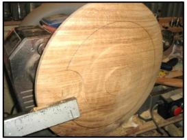
Here's the first of the petals being turned. Notice that the centre of the disc is way over from the centre of the petal, and with the centre of gravity so far over, I was not able to turn faster than 160rpm, I would have preferred 1,600rpm for such small features! Faster than 160rpm and the vibration is too much. I'm very grateful for the variable speed as the right speed is found by trial and error.
