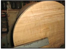
This is the front of the piece after shaping. There's a chucking spigot in the centre, a raised area which defines the corolla, and a pencil line 14½ inches from the opposite side to mark the centres for the petals. A strange way to measure it, you may say, but it ensures that the disc will not foul the lathe parts and fit the 29½ inch swing of the outrigger. The proportions look good and right, so carry on.
