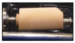
With larger diameter pieces, off setting in the above manner becomes more problematical, and a different method of holding is needed. The photograph on the left shows a 75mm diameter cylinder set on the lathe with a 10mm offset at the tailstock end.
