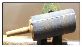
This simple and so useful sanding drum was made from a piece of holly, but any hardwood will do. I find 50mm diameter a convenient size. The wood is held between centres and the length of the drum section formed at the headstock end of the lathe to the width of the grit cloth available.
