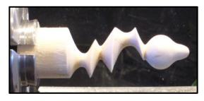
With a steady application of the tool, I use a  $^3/_8$ " spindle gouge, the cut will follow the bevel even though part of the cut is against the ghosting. Different shapes may be cut by varying the angle of cut and or the position and size of the waist
