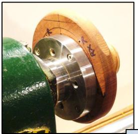
Note that one set of offset holes may be used to move the work to the left or to the right by rotating the faceplate halfway round on the connecting piece. The second photograph, left, shows the three pieces assembled on the lathe and offset to one side. The work piece is held centrally on the connecting piece. With this method, the work always remains parallel to the lathe axis. It maybe used for faceplate or spindle work, support from the tailstock is available if needed.
