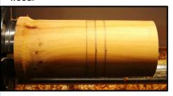
To position the handle I mark three lines, the start of the inside curve, the bottom of the cup and the wall thickness
