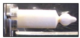
Off centre turning may be carried out by holding the work slightly off parallel to the lathe. This requires either a deep jaw chuck, cup chuck, split collet chuck or a jam chuck.
