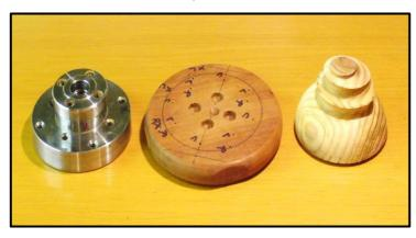
Off-centre work does not need a special off-centre chuck. One method of doing this is with a faceplate. The photograph, left. shows a faceplate. connecting piece, which does the off setting, and the work piece.
