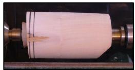
This will hold the work in the offset position, now return the work parallel to the lathe and form a larger (50mm) dovetail as indicated by the two parallel vertical lines. With the smaller dovetail and two lots of waste wood on the drive side, very deep jaws will be needed to hold the work.
