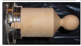
A standard deep jaw chuck may be used if the larger dovetail is cut to fit half-open jaws. This allows the work to project past the base of the jaws. It can be seen how the works fits into the chuck when being held parallel to the lathe by the larger dovetail.
