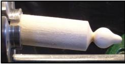
The movement of wood in the chuck is small. Turn the lathe by hand and check the waist will be where required and not too small. Looking straight down it will be formed on the centre line of the lathe. Always keep enough wood in the jaws so a good grip is obtained all the way around.
