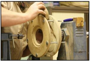
A jig was then produced to hold the bowl for the off centre turning. Marking out the piece for two different bowl sizes was facilitated using discs of wood to position and mark the centres for the two overlapping dishes. These centres would enable the tailstock to be used to position the bowl within the jig for cutting the dishes.
