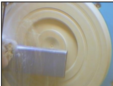
The inlay recess being cut.
