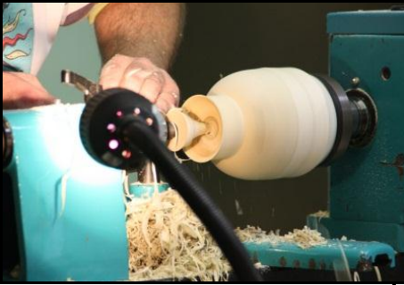
Hollowing for the legs, supported by the tail centre
