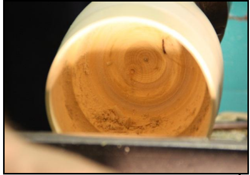
Hollowing the vase in layers
