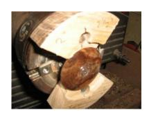
Note the centre mark on the jaw. Line up the piece and cut the centre chamfer. Again, do it slowly. Here I used a 3/8 " shallow fluted gouge. Polish with melamine and burnish.
