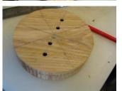
Now make a mark slightly off-centre, in line with the jaw-screw holes. I chose to offset mine by 3/16 inch.
