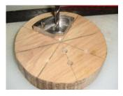
Take a bradpoint drill which snugly fits the screw holes in a chuck jaw and mark the screw positions on the marked side of the timber along the N-S line. Use the same drill to drill right through the wood.
