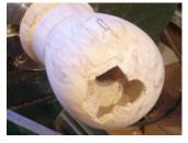
Always try the tool against the vessel before turning on the lathe. Make sure you have the right angle of presentation and note the angles required to get the tool in and out of the vessel. The straight bar scrapers will go straight in and out, but the swivel heads will take a bit more manoeuvring. Before inserting a swivel tool, ensure there is enough room inside the vessel, to contain it, and for it to work. Failure to do this may result in damage, as above.
