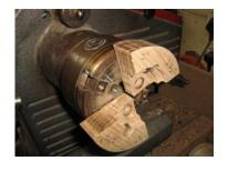
The finished jaws in place. Note that I've written the pendant diameters on them – I have two or three sets for different sizes, so writing the size on makes sense.
