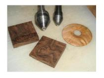
Now to make a pendant. I chose to use the Axminster ring drive and tailpiece. You can reverse the piece to access the chamfer more easily, and it's very effective at lining up the piece.
