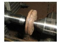
Place a blank between the centres, tighten up well and remove the corners. I used a 1/4" deep fluted gouge.
