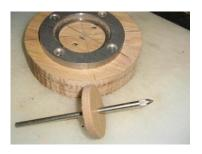
Centre a faceplate ring on that mark. See the gizmo in the foreground – place the point of the shaft on the mark, slide the MDF ring down the shaft and then place the faceplate ring over the MDF.
