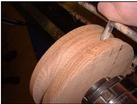
The cove being cut on the end grain.
