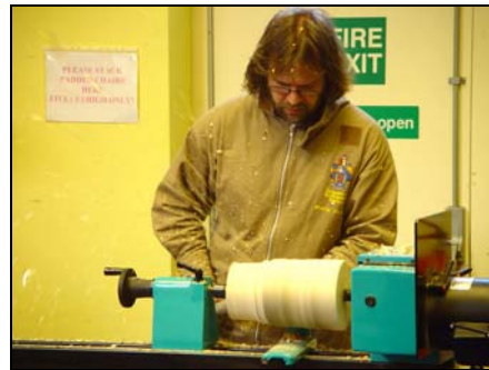
The wet log being roughed out
