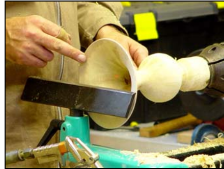
The hollowing completed
