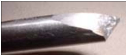
One of the bowl gouge grinds(flute at the top of the picture)
