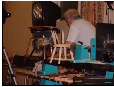
The chair being assembled on the lathe bed.
