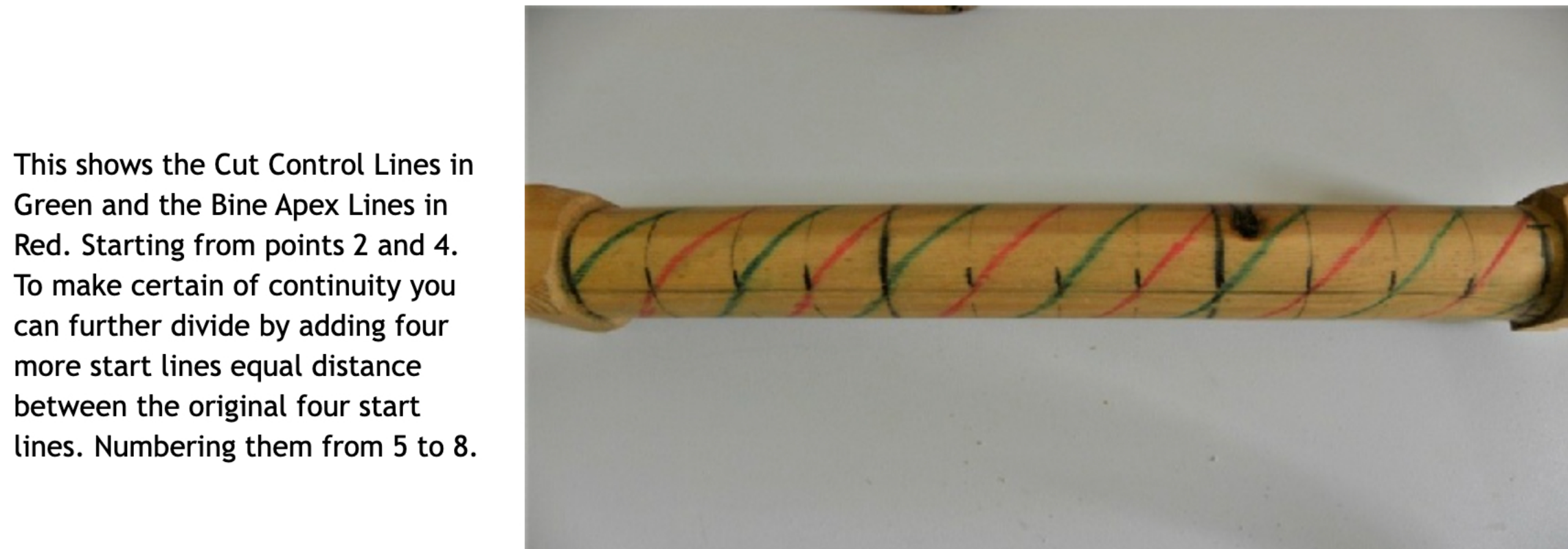
The next operation is to mark out the Cut Control Lines. I found that it was easier to use a piece of thin plastic to draw diagonally across the round starting from Start point taking it right to the end and then start again using start point three again right through to the end. I use different coloured for each line drawn.
