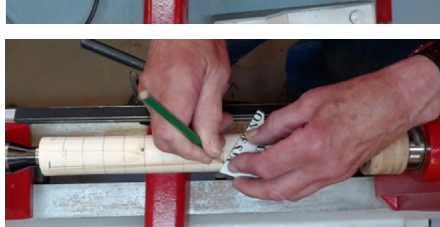
The next operation is to mark out the Cut Control Lines. I found that it was easier to use a piece of thin plastic to draw diagonally across the round starting from Start point taking it right to the end and then start again using start point three again right through to the end. I use different coloured for each line drawn.
