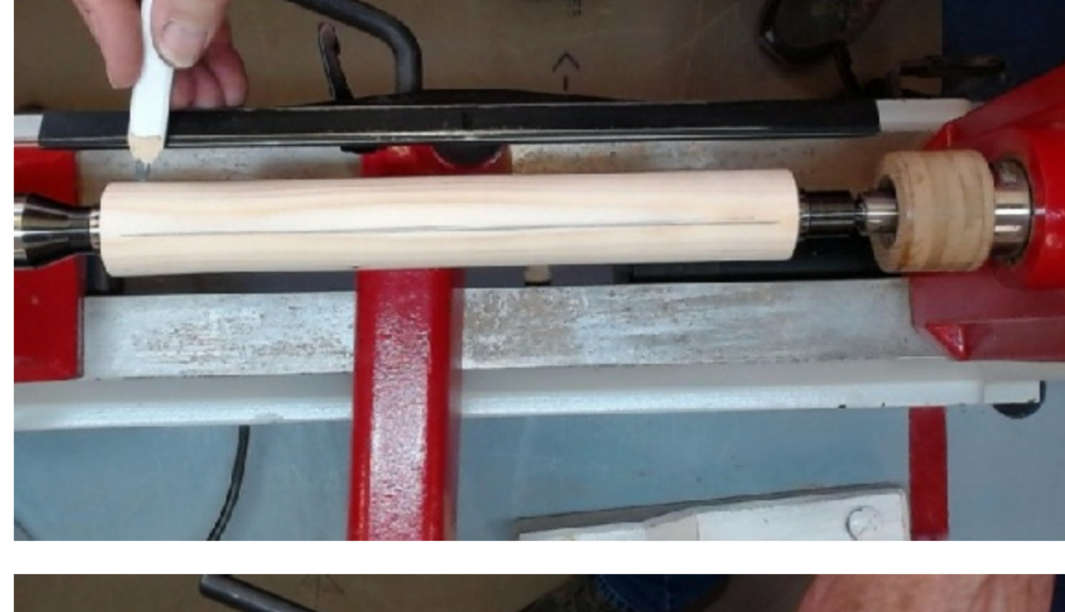
The four lines along the length will need to be numbered 1 to 4 on both ends these are the start points for marking out the Bines and Hollows.
