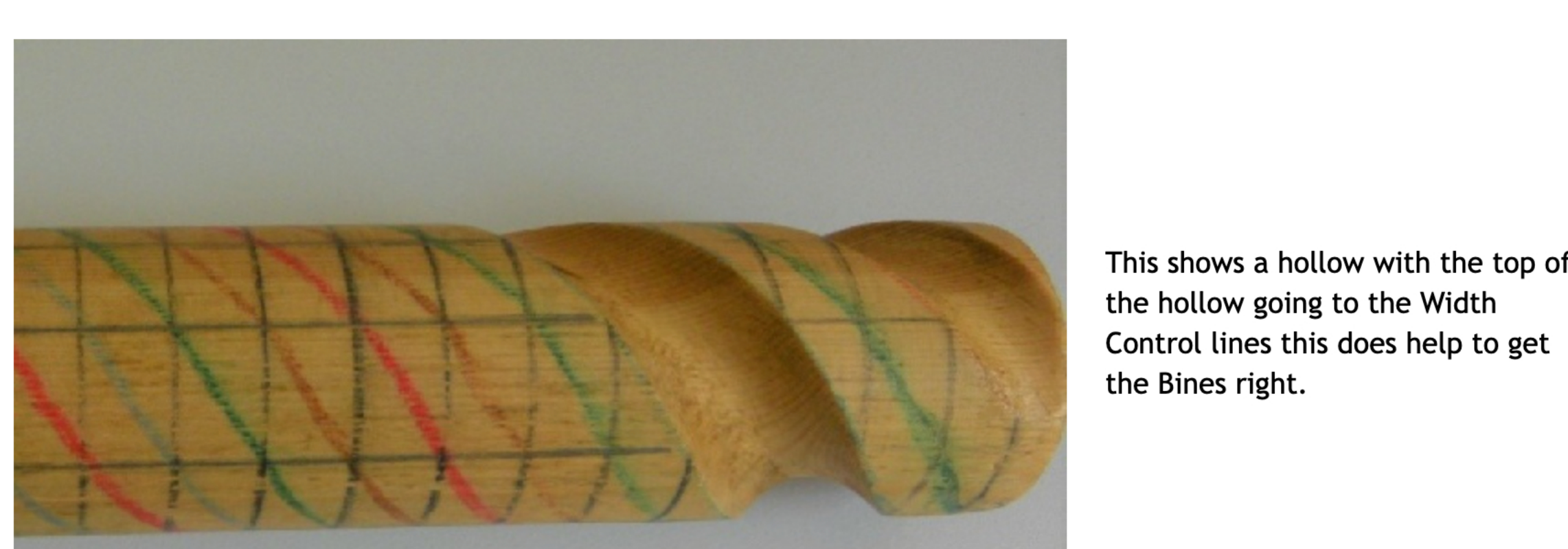
Using a flat Micro file you can start to form the round on the Bines until you meet the Bine Apex Lines. Continue to form the Twist until satisfied to allow you to start sanding.
