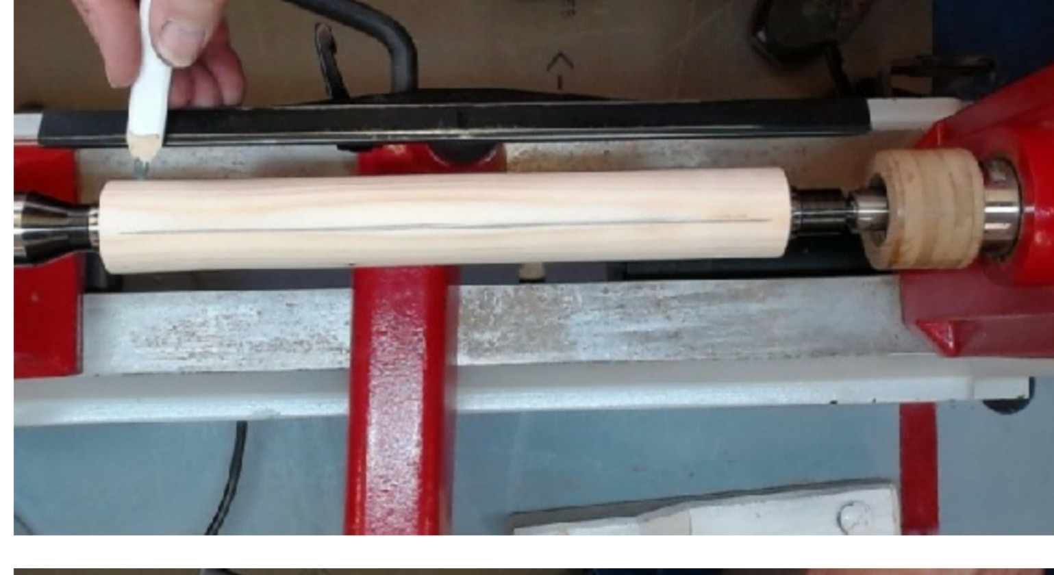
The four lines along the length will need to be numbered 1 to 4 on both ends these are the start points for marking out the Bines and Hollows.
