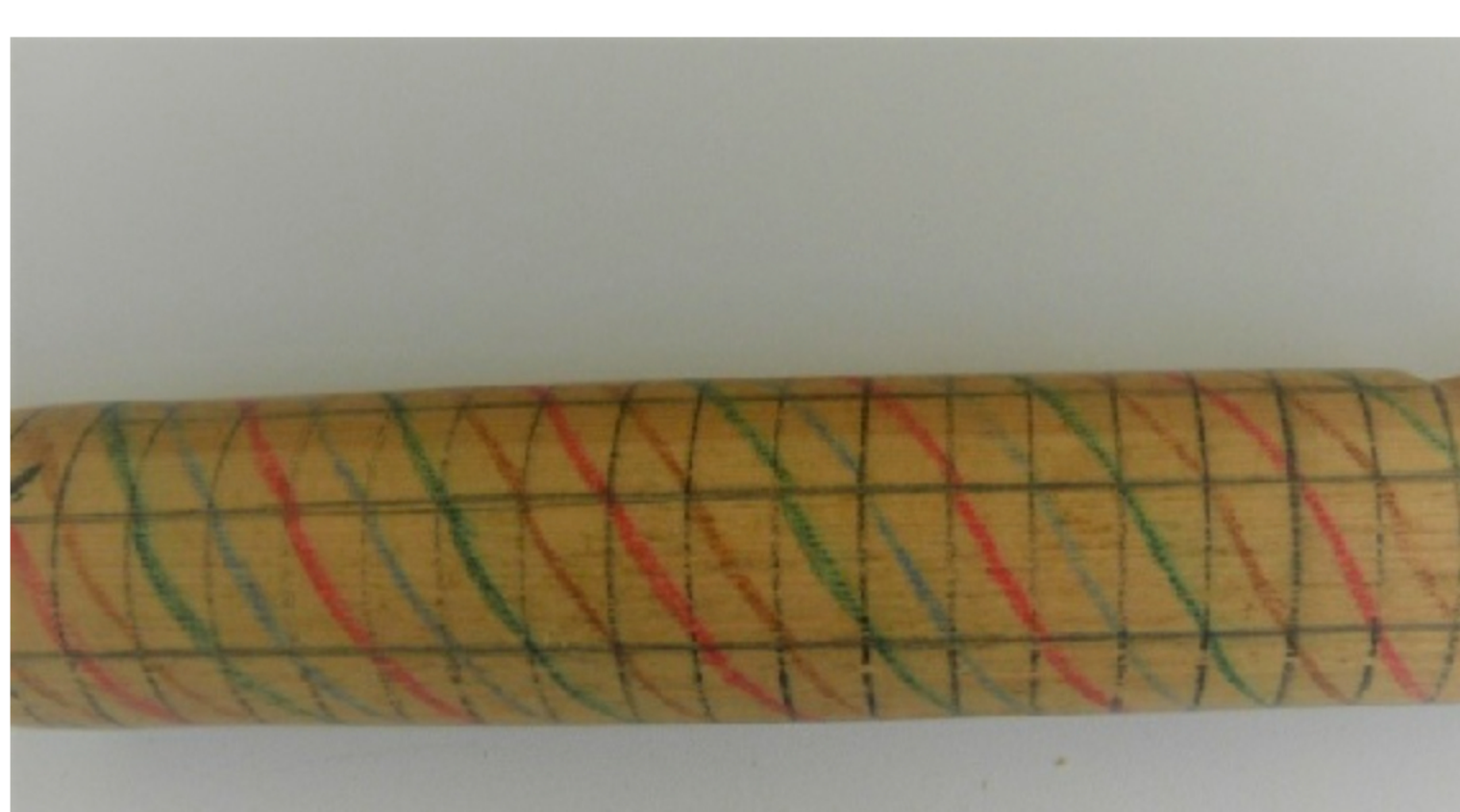
Here you can see that the Width Control Lines are coloured Blue and Brown and these of course start at points 5 to 8. Before you draw these width lines you will need to draw another circular line midway between each pair of pitch lines. These two photo's show left and right hand twists
