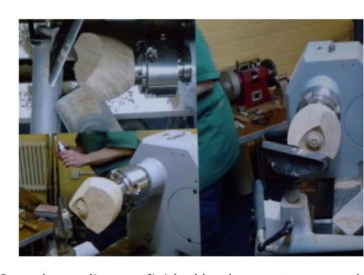
Once the sanding was finished he then went on to explain how to remove the foot of the bowl i.e.: - the original chucking point.
