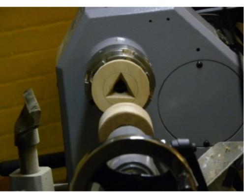
Mike explained that he found that using these chucking pieces the object blank was held much more securely than holding it between centres. Hopefully the next photo will make it clear has to how the piece was held.
