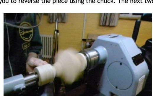
Once Mike was satisfied with the profile he showed how he would sand the item by putting the lathe into reverse (explaining to make certain that you had locked the chuck onto the spindle using the grub screw).
